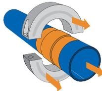
4. Secure both halves of the Ring using screws provided.
