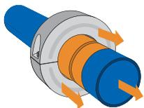
5. **IMPORTANT:** ensure that when installed there are no gaps between Ring and pipe and that Ring cannot move or turn around the pipe.
